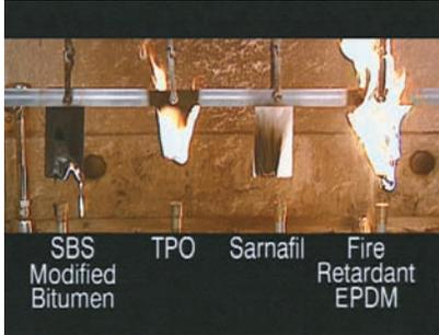
With Sarnafil, the fire stops when the flame is removed. With the other options, the alternative membranes continue to support combustion. With both the TPO and EPDM membranes, burning embers fall, which could spread the fire or contribute to internal fire.
